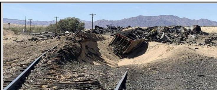
**March 27, 55 cars and 2 engines of a 154 car, 21,600 ton iron ore train derailed descending a 2.2% grade near Kelso, CA. Preliminary reports suggest that once the dynamic brakes shut down due to a technical malfunction, the air brakes were insufficient to control the train, which then became a runaway. The crew apparently managed to jump**
